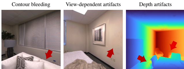
Fig. 9: Limitations of our method. Left: In some cases, Gaussians placed at object boundaries bleed to background which produces outline artifacts. Middle: Approaching the walls too much results in popping artifacts. Right: Sometimes, the inpainting latent diffusion model can hallucinate erratic content resulting in wrong depth estimates. Also, seamless depth blending is not always successful.
